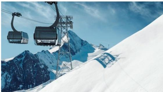
*A lift connection from the Maiskogel to the Kitzsteinhorn will become reality with the opening of the 3K K-connection in November 2019. Salzburg's first tri-cable gondola manufactured by Austrian company Doppelmayr is equipped with modern, custom-designed ATRIA cabins that will make their world premiere here on the Kitzsteinhorn.*
