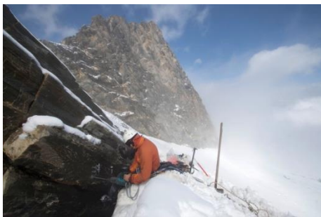
Drilling holes for temperature sensors
